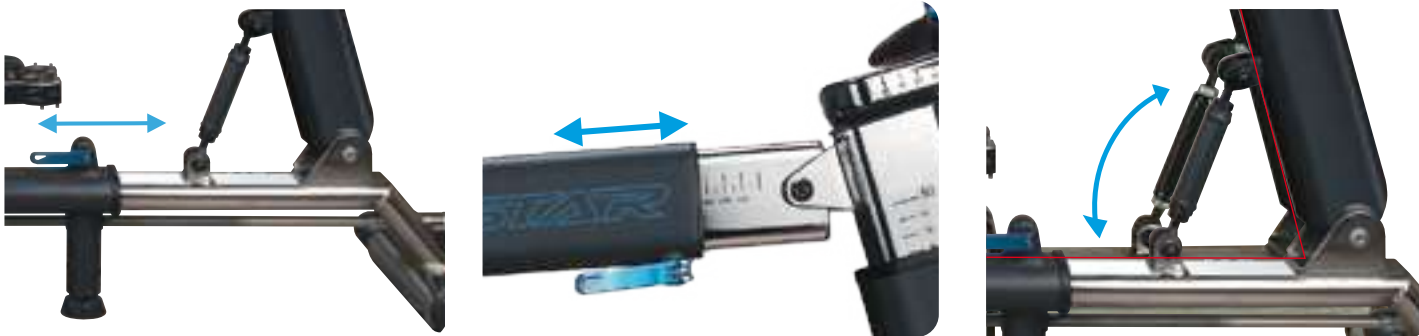
4 Top Tube adjustable 5 Top Tube adjustable 6 Head Tube angle adjustable
